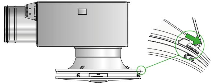
Locate the knob that protrudes from the diffuser face, slide the knob along the slot, the diffuser face is loose at the end position.
