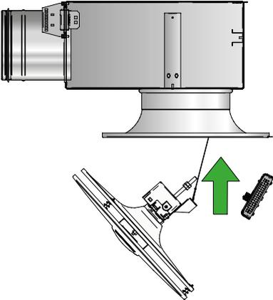
Reassemble, in the reverse order and connect hoses and contactors from WISE CU, see "Connection". Apply the new supplied QR codes over the existing QR codes on the product.
