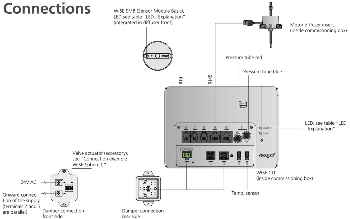
Figure 3. WISE Sphere C, connection.
