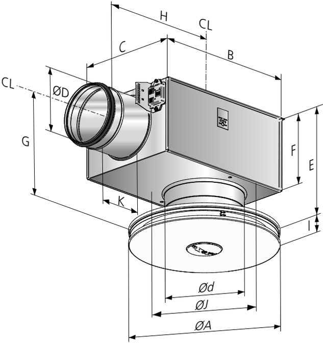
Figure 1. WISE Sphere C, dimensional figure.
