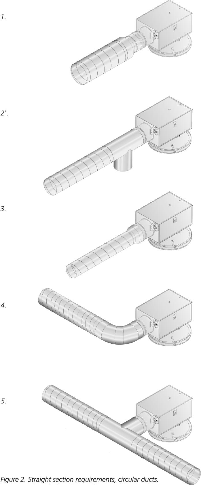
Figure 2. Straight section requirements, circular ducts.
