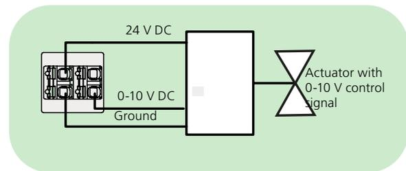
Connection of actuator with 0-10 V control signal.
