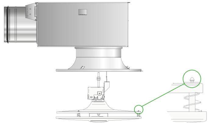
When refitting, fit the pin in the hole in the cone, press the diffuser face upwards at the same time as the knob is slid back.
