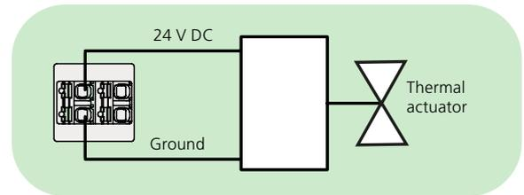
Connection of thermal actuator
